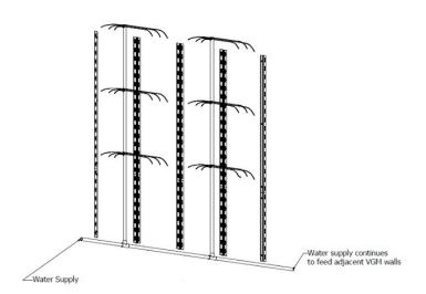
Once the units are hung, Tournesol recommends irrigating them with drip irrigation. Modules can be removed or attached independent of one another, should maintenance be necessary. New modules can be introduced to existing frames allowing replacements to be held in reserve.
